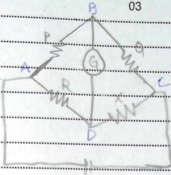
wheatstone Bridge has such construction as shown above with four resistors. The value of two resistors is known ( $P$  and  $Q$ ), value of one is variable ( $R$ ) and one is to be known ( $X$ ).
