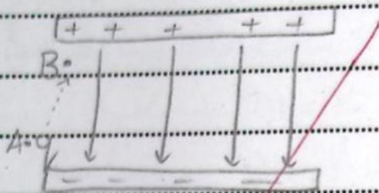
Consider the uniform electric field between two oppositely charged plates. Let A and B be the point in the electric field, the work done on the charge  $q$  that is present in the electric field is;
