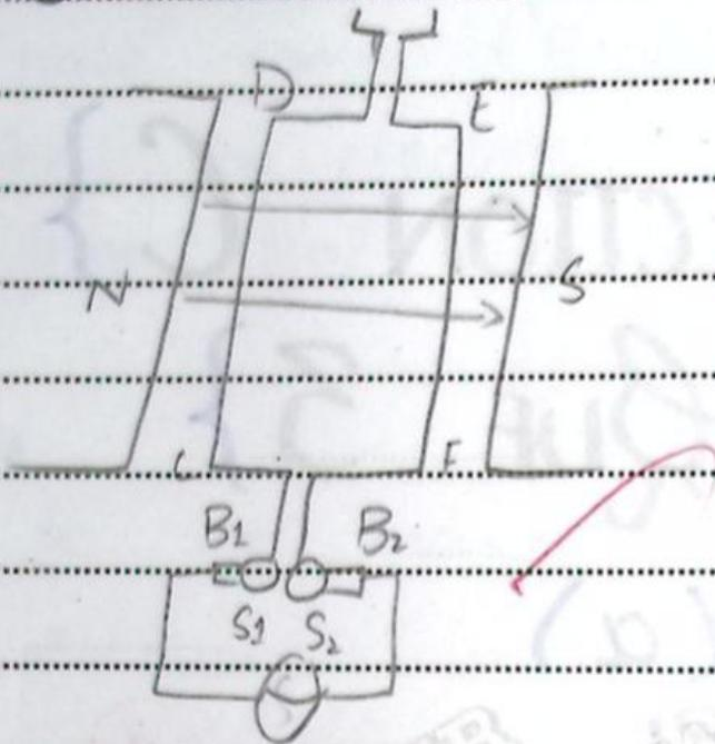
The AC generator consists of two permanent magnets, a coil that forms the loop CDEF, two slip rings  $S_1, S_2$  connected to the coil and with slip ring two carbon brushes are connected  $B_1$  and  $B_2$ .
