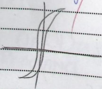
The hysteresis loop of soft material is narrow because when magnetizing force is applied, they easily get magnetized and when removed they easily get demagnetized.
