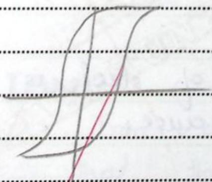
The hysteresis loop of hard material is wide because when magnetizing force is applied, they don't easily get magnetize & when removed
