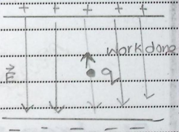
Negative sign shows that potential is increasing in opposite direction of electric field. This relationship is analogous to earth's gravitational field.
